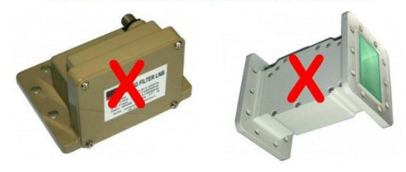
These low cost products omit proper cavity filter design to cut costs. Critical bandwidth and attenuation characteristics needed for proper operation does not exist. You end up with a partially functioning device that won't perform or meet your needs. Stay away from these.
